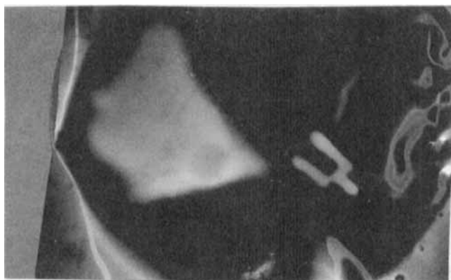
FIGURE 3. Thermal image of a surface of inhomogeneous body containing holes and inclusions of another material.
